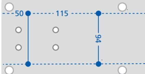
**For permanent mounting** on standard racks (up to 14,5cm in width) Choose the best position and opening direction that leaves enough space to the saddle. Take care that the cover can be opened easily. Press the 4 nuts into both brackets. Put screws through the holes that are ment for the **fix** Mounting (see diagramm) and screw them tightly with both brackets. If those holes don't fit for your carrier you can drill alternative holes Ø 6mm along the dashed lines.
